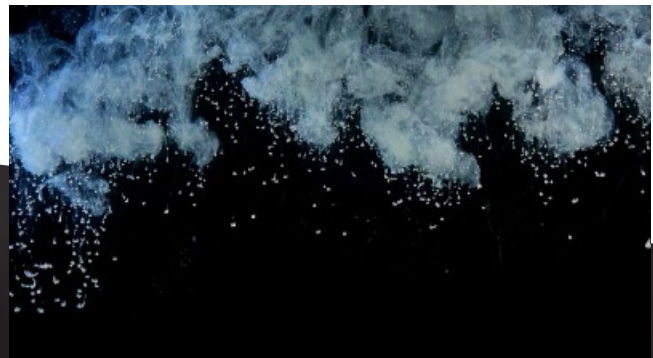
Example of a poor emulsion coalescence and flocculation occurring into water
