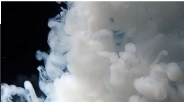
Example of a good emulsion blooming into water
